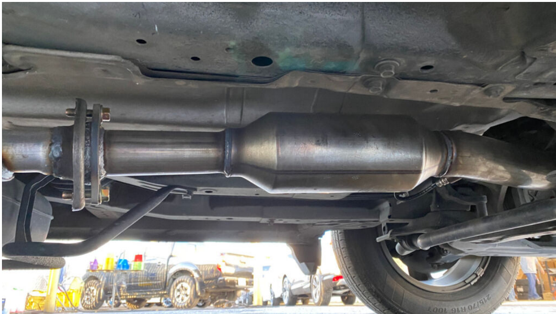
The ‘cat’ is the fat part in the exhaust pipe above.
